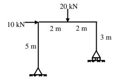
(b) Find out S.I. and K.I. for the structures as shown in figure below.
